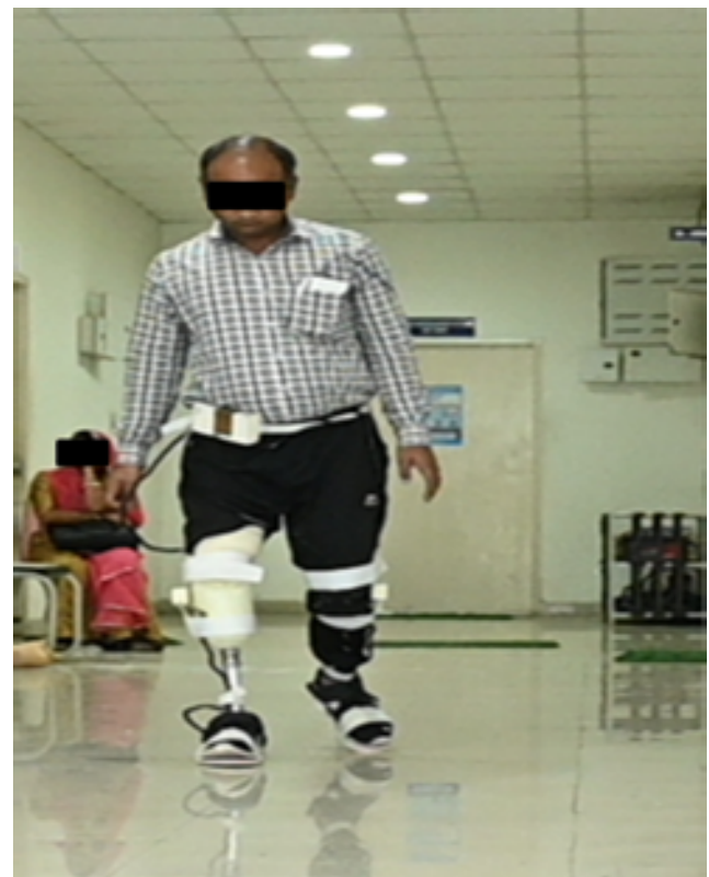
Fig. 2. Unilateral TT amputee wearing gait analysis setup.
